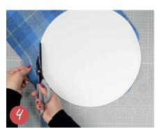
Cut off surplus covering by running a sharp knife along the edge of the panel or trim with scissors.
