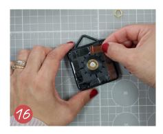
Remove the brass nut and washer, leave the rubber washer. Put double-sided Tesa tape around the clock housing and then remove release paper.
