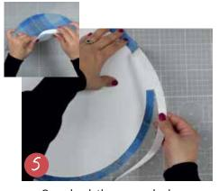
Snap back the creased edges around the panel until the PVC breaks, then remove.
