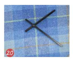
Fit the Minute Hand Repeat the process with the minute hand, again ensuring it is pointing to the 12 o'clock position.
